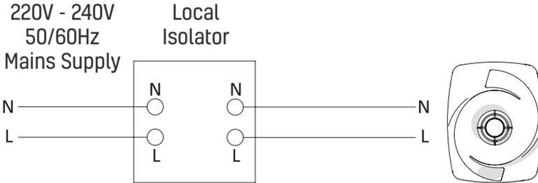
Connect the local isolator to the Mains as part of the fixed wiring. Connect the N and L connectors of the fan power cable to the local isolator.
