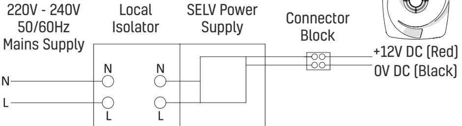
The red 12V cable from the unit must be connected to the red cable on the SELV power supply using the supplied terminal block. The black 12V cable from the unit must be connected to the black cable on the SELV power supply using the supplied terminal block.
