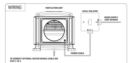
The local isolator must be connected to the mains as part of the fixed wiring. Connect the N, L and E cores of the power cable to the matching terminals on the local isolator.
