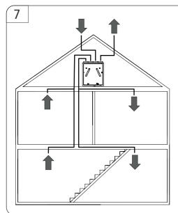
Ductwork should be fitted in accordance with the Domestic Ventilation Compliance Guide. (Example RH unit configuration shown).
