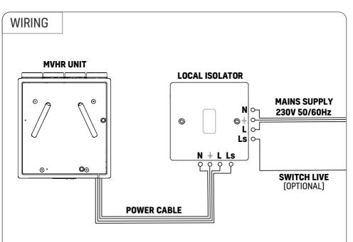
The local isolator must be connected to the mains as part of the fixed wiring. Connect the cores of the power cable to the matching terminals on the local isolator (3A fuse spur or similar).
