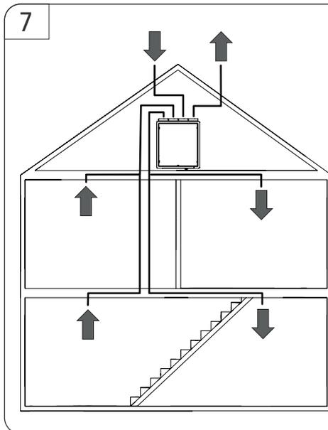
Ductwork should be fitted in accordance with the Domestic Ventilation Compliance Guide. [Example RH unit configuration shown].
